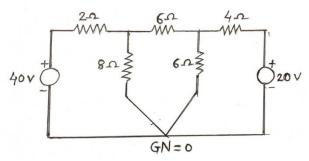
Apply KCL to  $V_1: 19v_1 - 4v_2 = 480$ ------(4) Apply KCL to  $V_2: -2v_1 + 7v_2 = 60$ ------(5)
