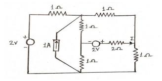
Solution: By using I-shift rule we can redraw the given network
