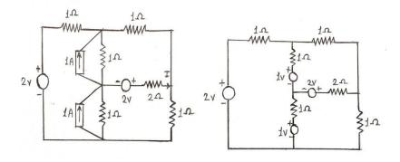
By converting current source into voltage source
