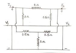
Solution: By using Y-parameter
